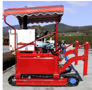
Photo 3. Riding-type tea field management machine (Medium pruning, Fertilization, Deep plowing) The provision of these photos is Matsumoto-kiko Co., Ltd. ( http://matsumotokiko.co.jp/index.html )
