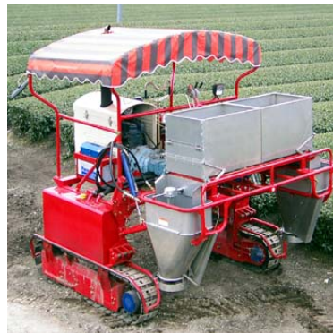
Photo 3. Riding-type tea field management machine (Medium pruning, Fertilization, Deep plowing) The provision of these photos is Matsumoto-kiko Co., Ltd. ( http://matsumotokiko.co.jp/index.html )
