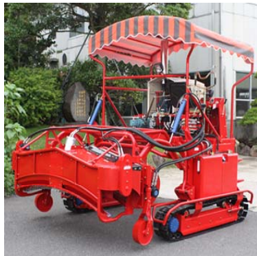
Photo 3. Riding-type tea field management machine (Medium pruning, Fertilization, Deep plowing) The provision of these photos is Matsumoto-kiko Co., Ltd. ( http://matsumotokiko.co.jp/index.html )
