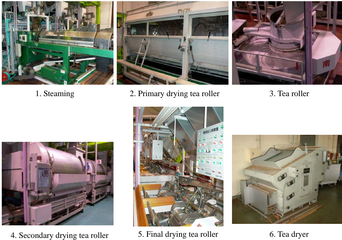
Figure 5 Japanese green tea ('sencha') manufacturing machines
