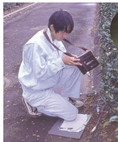
Check of nutrient status in tea fields with the EC sensor
