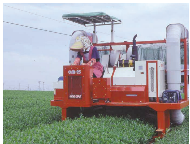
Riding-type plucking machine
